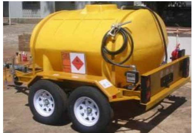
1500L POLYETHYLENE TANK WITH 12V DC PUMP & MECHANICAL FLOW METER
